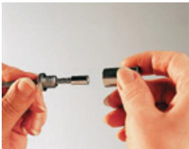
Montage mittels ASS Zylinderterminal
